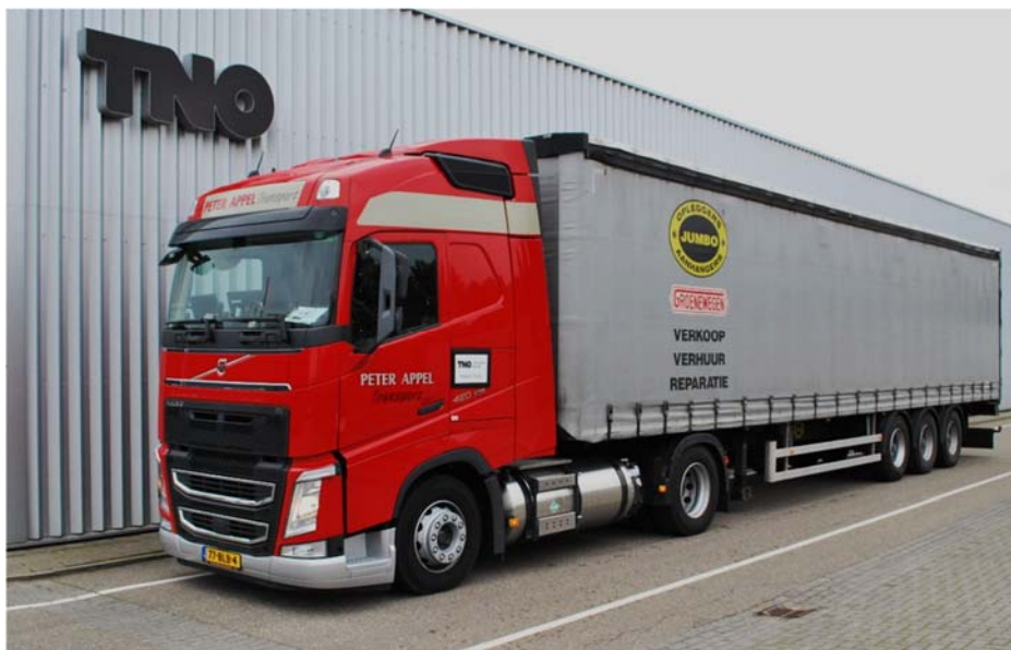
Figure 1: The test subject, a Volvo FH420 tractor with a Euro VI step C certified '1A' HDDF heavy-duty dual-fuel engine with LNG as the main fuel.
